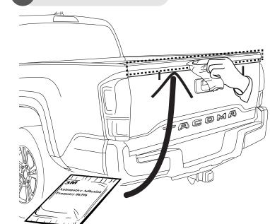
A full surface contact between tape and substrate is decisive for good adhesion performance. Contact is achieved by applying pressure. In practice a pressure between 40 and 50 N/cm<sup>2</sup> is usually needed and an application temperature between 25 and 45 °C or 77 and 113 °F is also necessary. During application, add-on parts and tapes must have the similar temperature.
